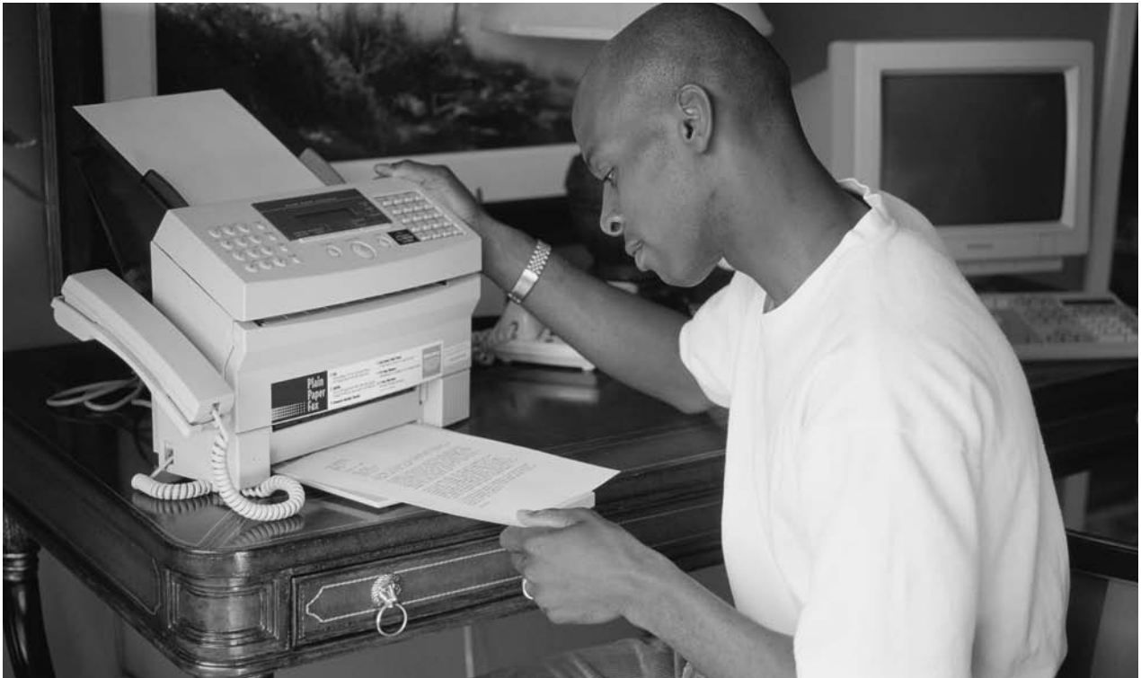
The sending fax machine uses a sensor to scan the document and to convert the pattern of black and white elements into a code. The receiving machine decodes and uncompresses the information and prints it.
